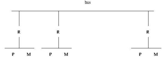
Each P/M/R set here is called a **processing element** (PE). Note that each PE has its own local bus, and is also connected to the global bus via R, the router.
